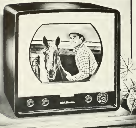
The "Talbot", table-model receiver with a 16-inch kinescope, is housed in a maroon metal cabinet
